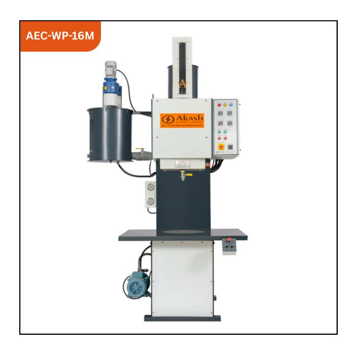
Machine Name: Manual Wax Injection Press Hydraulic
